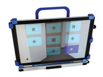
The A13J is a lightweight alternative drive control you can use with your eyes. This device is designed for people who can no longer use the joystick on their powered wheelchair and do not have a supported eye gaze device.
